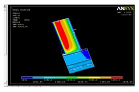
Thermal Flux for inconel 625 alloy is 0.63026 w/mm2
