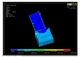
Thermal Flux for Haste Alloy X is 1.07965 W/mm<sup>2</sup>
