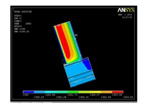
Thermal Flux for Haste Alloy X is 0.490218 W/mm<sup>2</sup>
