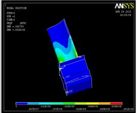
Deformation for Haste Alloy X is 0.1670 mm
