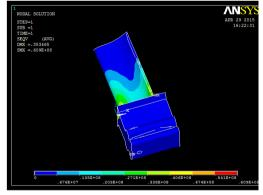
Von Misses Stress for Titanium Alloy X is  $609 N/mm^2$
