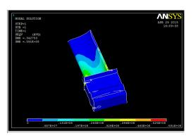
Deformation for Stainless Steel Allloy is 0.14473 mm
