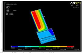
Thermal Flux for Haste Alloy X is 0.747055 W/mm<sup>2</sup>
